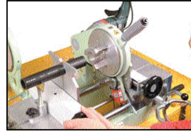
Preparing to peel the pipe
