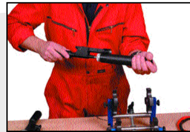
Peeling the pipe
