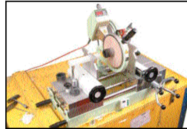
The heating element is moved into place
