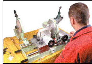
Peeling the pipe
