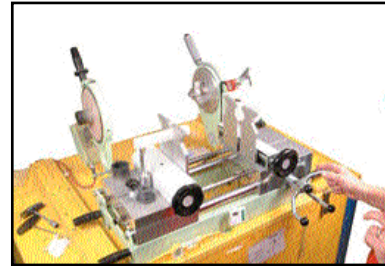
The fitting is mounted in the clamps
