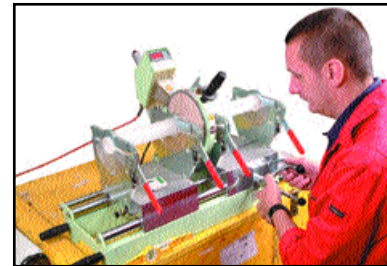
Preparing to remove heating element
