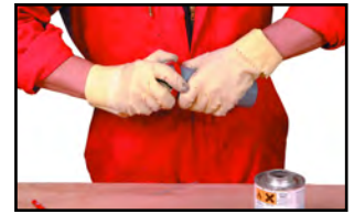
Chamfering the pipe
