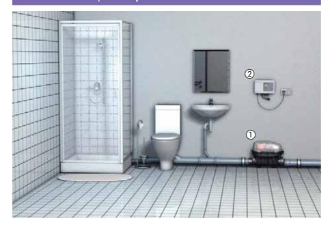
Function and range of application are identical to the system described above. The installation of the Pumpfix F(1) is even easier in this case if the wastewater pipe is routed exposed across the basement floor. The Comfort control unit 2 with SDS is part of the scope of supply here, too, so that safe system operation is guaranteed at all times. A low-cost investment for backwater protection in the basement compared with the property and building damage caused by basements flooded by backwater.
