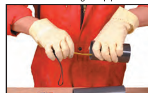
Measuring the insertion depth
