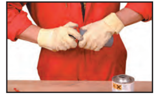
Chamfering the pipe
