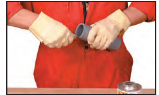
Removing the internal burr
