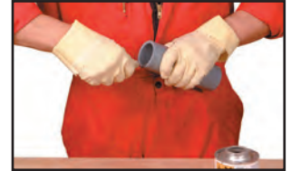
Removing the internal burr
