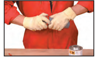
Chamfering the pipe
